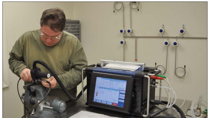
A Weldship employee demonstrates the art of orbital welding at their facility in Bethlehem, PA.
