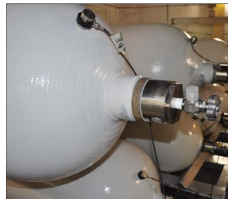
Acoustic emission testing in progress at Weldship's facility in Bethlehem, PA.
