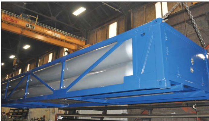
An ISO container, manufactured to hold an electronic grade gas, is being lowered onto a truck to be shipped overseas.
